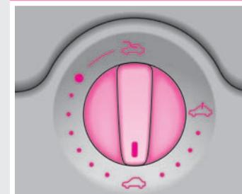
The sliding/tilting roof is opened and closed by means of a switch when the ignition is on.
